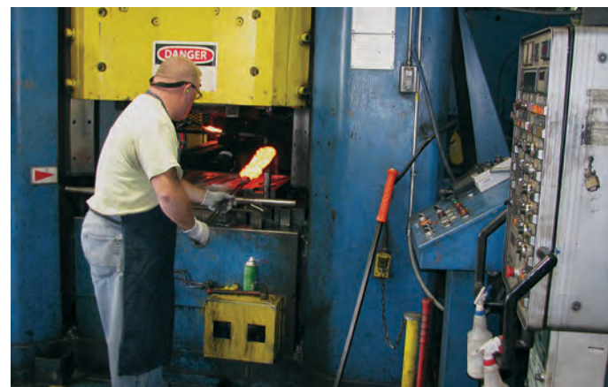
An operator forges a large tool out of steel on the forge press at the Snap-on plant in Elizabethton.
